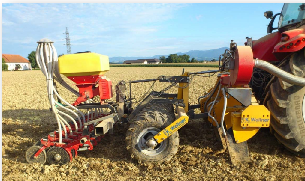
Seeding in rows with disc shares together with sub soiling SEEDING DATE: 15.08.2012
