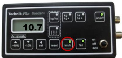
7. Press the „km/h“ button. The display show the actual speed in km/h.
