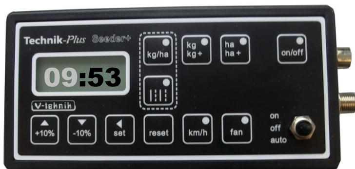
**Startup** = It is after connecting the SEEDER+ unit with the battery. On the display is shown a dashed line and one LED after the other starts to shine.
