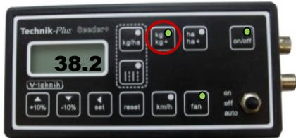
5. Press the „kg/kg+“ button. The display shows the previously output amount in kg.
